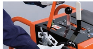
MANUAL OR HYDRAULIC RAISE & LOWER THE BLADE
