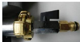
DUAL WATER-INLET AND DUST-COLLECTOR CONNECTOR
